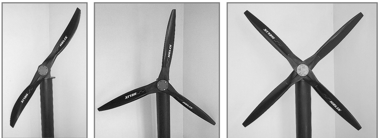
Figure 1: 2-, 3- and 4-blade propeller of type H50F
