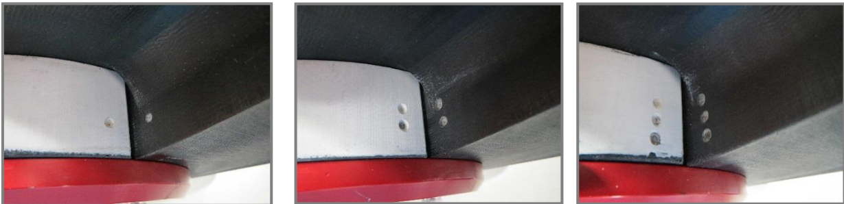
Figure 3: Blade positioning by milling marks.
