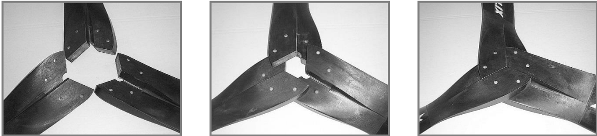
Figure 4: Mounting of the 3-blade propeller (here without position numbers)
