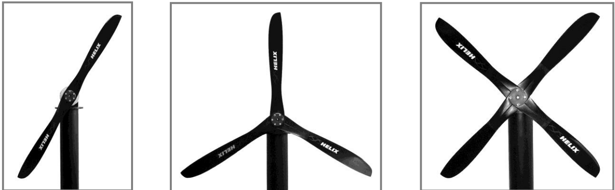
Figure 1, 2 and 3: 2-, 3- and 4-blade Propeller of Type H40F
