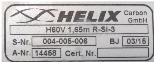
Certificated propellers are identified in the type label with a suitable Cert. Number.
