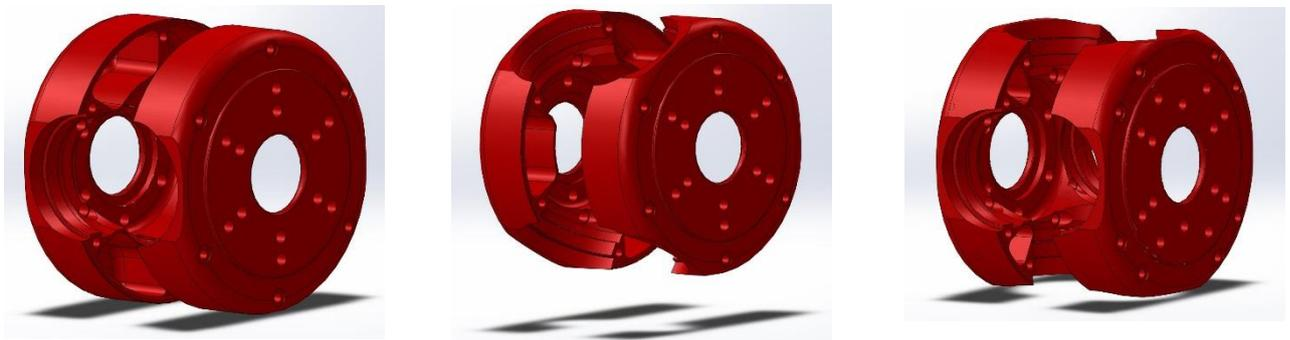
**Figure 2:** 2-Blade, 3-Blade and 4-blade hub
