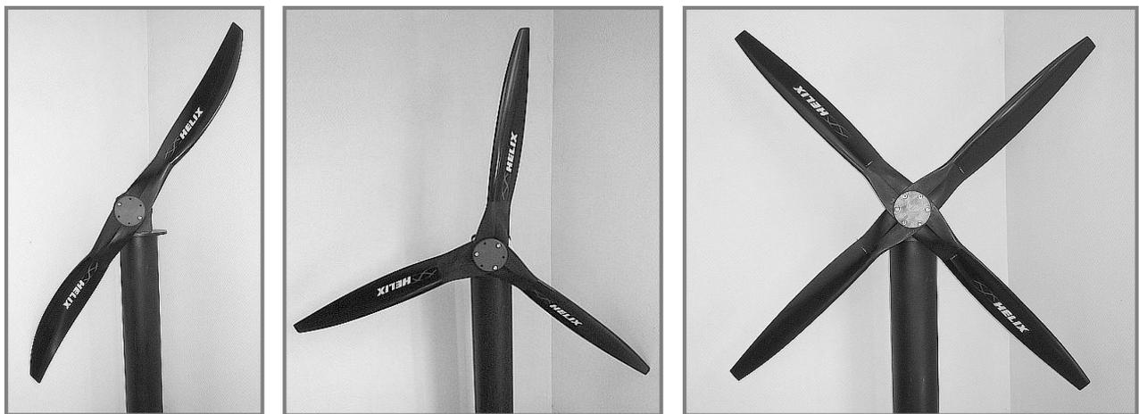
**Figure 1:** 2-, 3- and 4-blade propeller of type H50F
