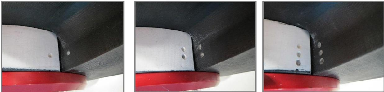
**Figure 3:** Blade positioning by milling marks.
