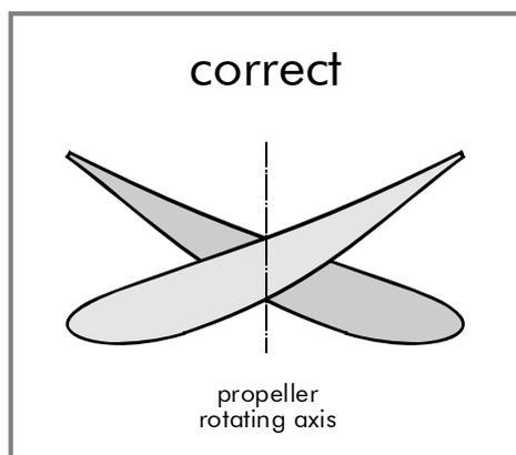
**Sketch 1:** Correct position of the propeller blades
