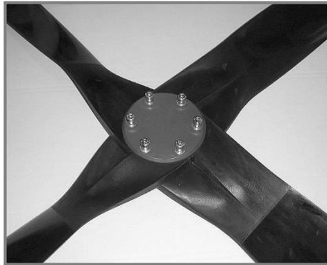
**Figure 7:** 4-blade propeller with mounted front plate
